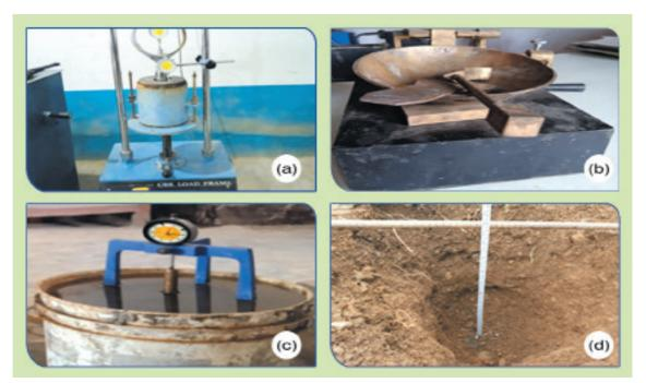
Figure 1: Sampling and Testing. (a) CBR testing of samples, (b) Casagrande testing devices, (c) Soaking of Sample, (d) Sample taking from site,
